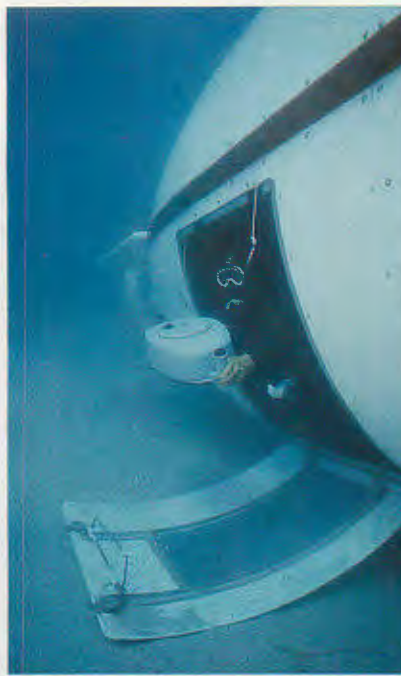
Diver in bubbleless rebreathing apparatus deploys from minisub with limpet mine.
